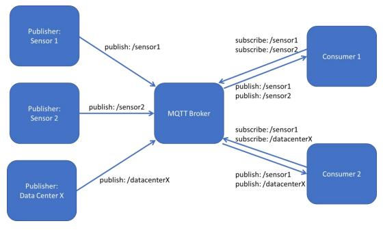
Figure 5: Schematic overview of MQTT
